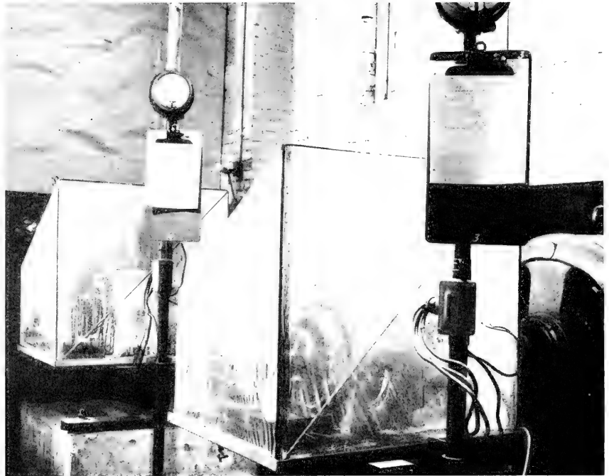
1. Silicone-insulated test motors are operated alternately at temperatures up to 310 degrees centigrade and exposed to 100 percent relative humidity. Tests show that moisture is excluded after thousands of hours of thermal aging.
